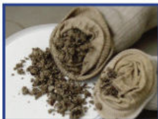
Scum collected in a sock during a boil out with BIOMatic
