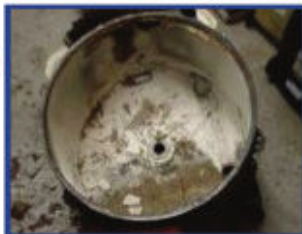
Washing machine outer drum before boil out filled with scum
